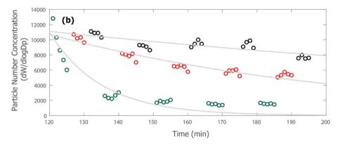
Fig. 2 Measuring particulate matter decay across three rooms with a HEPA purifier active by switching the inlet hose on the SMPS at five-minute intervals. (a) Shows an example time-series and how this varies for three rooms and (b) shows an example exponential fit from which a rate of decay can be calculated.
