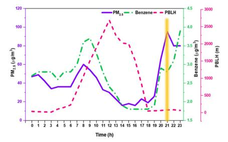
Fig. 4 High resolution monitoring data (averaged over 15 min interval) of PM<sub>2.5</sub> and benzene with PBLH on April 5, 2020. The yellow glow line highlights the lamp event at 21:00 h.
