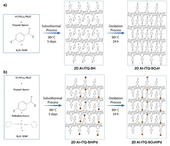
Fig. 7 Representation of metalorganic materials synthesis: (a) Al-ITQ-SH and Al-ITQ-SO<sub>3</sub>H and (b) Al-ITQ-SH/Pd and Al-ITQ-SO<sub>3</sub>H/Pd. The dark spheres represent the palladium nanoparticles. Reproduced from ref. 61 with permission from the Royal Society of Chemistry
