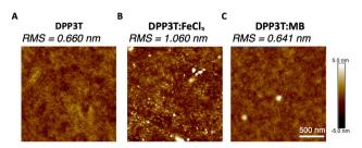
Fig. 2 AFM images of the DPP3T (A) pristine film surface, (B) doped with FeCl<sub>3</sub> and (C) doped with Magic Blue with RMS values of each of the films.
