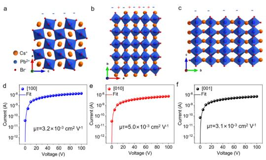
Fig. 2 (a-c) Arrangement of [PbBr<sub>6</sub>]<sup>4-</sup> octahedrons in the CsPbBr<sub>3</sub> crystal structure, and (d-f) photocurrent fitting curves of the [100], [010], and [001] wafers of CsPbBr₃ crystal
