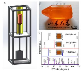
Fig. 1 (a) Schematic diagram of the vertical Bridgman furnace. (b) Photograph of an as-grown CsPbBr<sub>3</sub> single crystal. (c) XRD patterns of the (100), (010), and (001) wafers. The insets are photographs of the processed and polished wafers.
