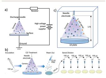
**Fig. 1** (a) Schematic of the CD treatment setup; (b) procedure of the sterilization experiments, including inoculation with microorganisms, CD treatment, washing out surviving colonies, serial dilution using PBS, and plating; (c) schematic of CD air sterilization test setup.
