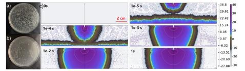
Fig. 4 Cultured LB plates of E. coli-contaminated air (a) without and (b) after 7.5 minutes of CD treatment at 25 kV and 0.05 mA; (c) the electron density distribution map changed over time after the corona was turned on.
