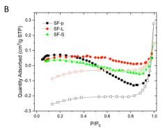
Fig. 6 Isotherms obtained from sphene derived samples showing negligible or no gas adsorption. (A) Granules derived from 3D printed sphene blocks: large (SB-L); small (SB-S); pulverized (SB-p). (B) Granules from sphene foam blocks: large (SF-L); small (SF-S); pulverized (SF-p).
