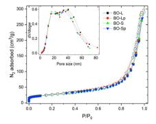
Fig. 5 Isotherms of Bio-oss® granules large (BO-L); small (BO-S); pulverized from BO-L (BO-Lp) and from BO-S (BO-Sp). Open symbols are for desorption. The inset graph represents the pore size distribution, evaluated using the BJH model in desorption.
