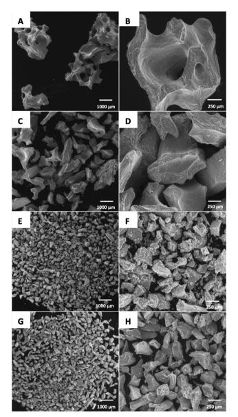
Fig. 1 SEM images of the investigated Bio-oss® granules: (A) and (B) large (BO-L); (C) and (D) small (BO-S); (E) and (F) pulverized from BO-L (BO-Lp); (G) and (H) pulverized from BO-S (BO-Sp).
