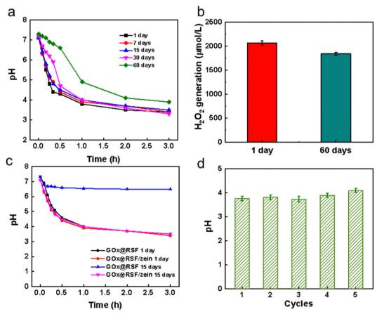
Fig. 3 The stability of GOx@RSF/zein nanospheres. (a) pH change with the reaction time after a different storage period (glucose solution: 1 mg mL<sup>-1</sup>), (b) H<sub>2</sub>O<sub>2</sub> generation after 1 day and 60 days of storage, (c) pH change compared with GOx@RSF nanospheres, and (d) pH value during different cycles.
