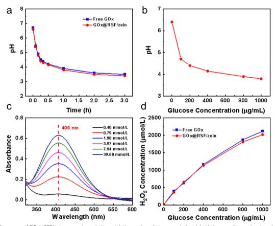
Fig. 2 The performance of GOx@RSF/zein nanospheres in the catalytic reaction of glucose solution. (a) pH change with reaction time (glucose solution: 1 mg mL<sup>-1</sup>), (b) pH changes with glucose concentration (reaction time: 1 h), (c) UV-vis spectra of Ti(v)O<sub>2</sub>SO<sub>4</sub> solution under different H<sub>2</sub>O<sub>2</sub> concentrations, and (d) H<sub>2</sub>O<sub>2</sub> generated in glucose solution under different concentrations (reaction time: 1 h).
