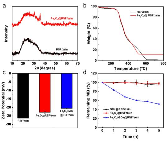
Fig. 4 The characterization of Fe<sub>3</sub>O<sub>4</sub>@RSF/zein and Fe<sub>3</sub>O<sub>4</sub>/GOx@RSF/zein nanospheres. (a) XRD pattern, (b) TGA curve, (c) zeta potential, and (d) degradation of methylene blue.
