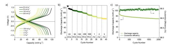
Fig. 2 (a) Galvanostatic profiles at different current rates and (b) discharge capacity of (+)DAAQ-TFP-COF||DAAQ-TFP-COF-M(-) symmetric cells during rate capability test. (c) Cycling stability and coulombic efficiency of (+)DAAQ-TFP-COF||DAAQ-TFP-COF-M(-) symmetric cells during long-term cycling at a current density of 500 mA  $g^{-1}$ .
