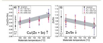
Fig. 4 (a) Cu/(Zn + Sn) and (b) Zn/Sn compositional ratios of the CZTS MGP crystals depending on the post-annealing regime as determined by EDX. Reproduced from ref. 34 with permission from Elsevier B.V., Copyright 2022.
