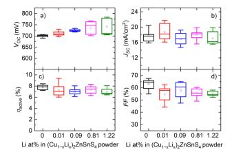
Fig. 11 Box-plot diagram of CZTS solar cell parameters (a) open circuit voltage  $(V_{OC})$ , (b) current density  $(J_{SC})$ , (c) efficiency  $(\eta_{active})$  and (d) fill factor (FF) with different Li concentrations in the CZTS powder. Reproduced from ref. 32 with permission from Elsevier B.V., Copyright 2023
