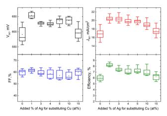
Fig. 9 Box plots of open circuit voltage, short-circuit current density, fill factor and efficiency of MGL solar cells fabricated from ACZCTS monograin powders with different added Ag content with respect to Cu. Reproduced from ref. 28 with permission from the Royal Society of Chemistry, Copyright 2019.
