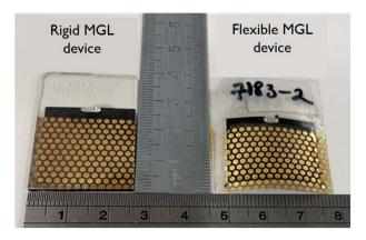
Fig. 13 MGL device on the glass substrate (left) and on the polymer substrate (right)
