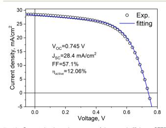
Fig. 12 Current density-voltage curve of the record efficiency CZTS MGL solar cell.
