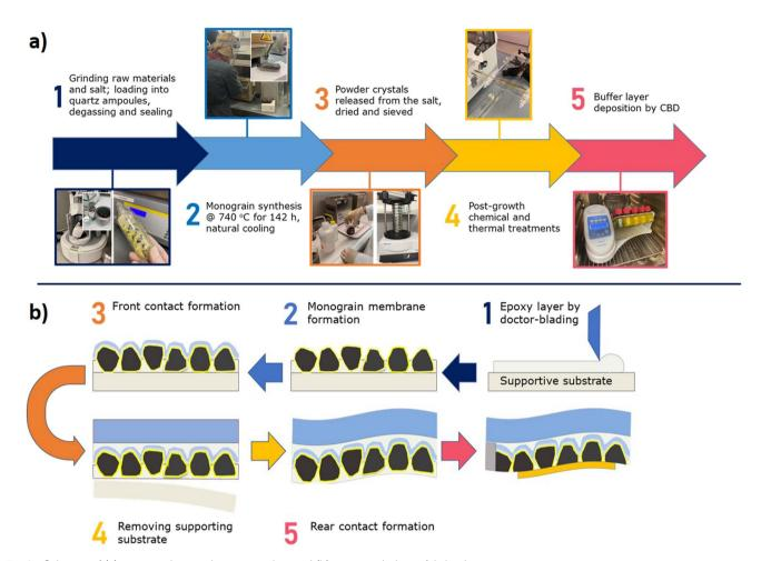
Fig. 2 Scheme of (a) monograin powder preparation and (b) monograin layer fabrication.
