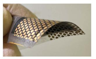
Fig. 1 Photo of a flexible CZTS monograin layer device with size of 2.5 cm  $\times$  2.5 cm.
