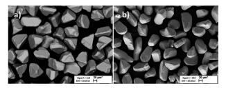
Fig. 6 SEM images of  $(Cu_{1-x} Ag_x)_{1.85}(Zn_{0.8}Cd_{0.2})_{1.1}SnS_4$  monograin powder crystals: (a) x = 0 and (b) x = 0.15. Reproduced from ref. 28 with permission from the Royal Society of Chemistry, Copyright 2019.
