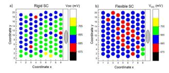
Fig. 14 Map of the  $V_{\rm OC}$  over the 2.5 cm  $\times$  2.5 cm area obtained from (a) the rigid MGL solar cell and (b) flexible MGL solar cell (contact size  $0.018 \text{ mm}^2$
