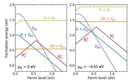
Fig. 4 Formation energies as a function of Fermi level for hydrogen interstitial ( $H_i$ ) and hydrogen-vacancy complexes, including the H +  $V_{7n}$ , 2H +  $V_{ZP}$ , and  $H + V_P$ , in  $Zn_3P_2$ , under Zn-poor/P-rich condition and at two different chemical potentials of  $H(\mu_H)$ : the H-rich limit  $\mu_H = 0$  eV (left panel) and a lower  $\mu_H$  at -0.45 eV (right panel). For comparison the formation energy of  $V_{Zn}$  is also depicted.
