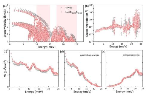
Fig. 4 Calculated group velocity (a) and scattering rate (b) *versus* the energy of phonon modes for LuNiSb and LuNiSb<sub>0.875</sub>Sn<sub>0.125</sub>. Energy dependence of p-p scattering phase space (c), the absorption process (d) and emission process (e).
