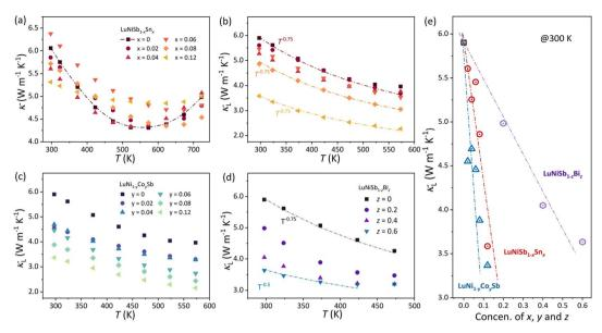
Fig. 2 Temperature dependence of the  $\kappa$  (a) and  $\kappa_L$  (b) for LuNiSb<sub>1-z</sub>Sn<sub>z</sub>. The temperature-dependent  $\kappa_L$  of (c) LuNi<sub>1-y</sub>Co<sub>y</sub>Sb and (d) LuNiSb<sub>1-z</sub>Bi<sub>z</sub>. (e) Nominal doping of alloying concentration dependence of  $\kappa_L$  for LuNiSb<sub>1-z</sub>Sn<sub>z</sub>, LuNi<sub>1-y</sub>Co<sub>y</sub>Sb and LuNiSb<sub>1-z</sub>Bi<sub>z</sub>.
