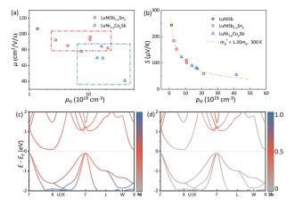
Fig. 6 (a)  $\mu_{\rm H}$  as a function of  $p_{\rm H}$  and (b) the Pisarenko curves with  $m_{\rm d}^* \approx$ 1.2  $m_e$  for LuNiSb<sub>1-x</sub>Sn<sub>x</sub> and LuNi<sub>1-y</sub>Co<sub>y</sub>Sb at room temperature. The projected band structure of (c) Ni and (d) Sb for LuNiSb.
