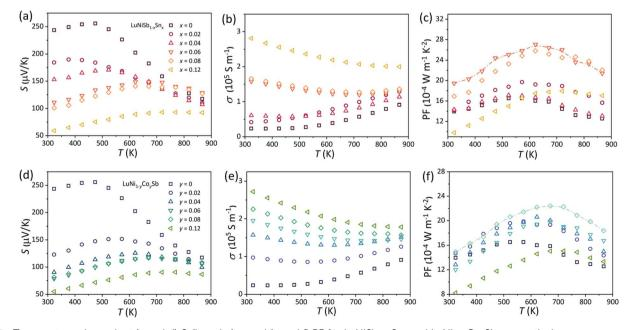
Fig. 5 Temperature-dependent (a and d)  $S_r$  (b and e)  $\sigma_r$  and (c and f) PF for LuNiSb<sub>1-x</sub>Sn<sub>x</sub> and LuNi<sub>1-y</sub>Co<sub>y</sub>Sb, respectively.
