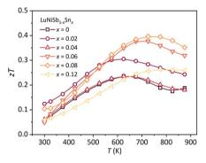
Fig. 7 Temperature dependence of zT for LuNiSb<sub>1-x</sub>Sn<sub>x</sub>.
