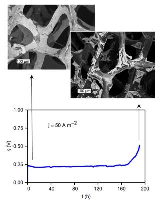
Fig. 7 CP showing the stability of a CoO<sub>x</sub>/RVC film under a current of 50 A m<sup>-2</sup> with micrographs of the material at its initial state, and after failure. The scale bars are 100 µm.
