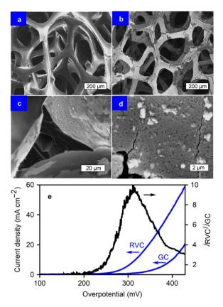
Fig. 6 SEM images of RVC electrodes (un-)coated with CoO<sub>x</sub>. (a) Pristine RVC. (b-d) Progressively higher magnification of CoO<sub>x</sub> films on RVC after 30 deposition cycles and electrochemical conditioning. (c) Cross section of the CoO<sub>x</sub> films on RVC.
