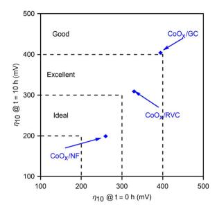
Fig. 10 Parametric plot of the overpotentials at a current density of 10 mA cm $^{-2}$  at the start of polarization (x-axis) and at t=10 h (y-axis) for three  $CoO_x$  films deposited on the three substrates: GC, RVC and NF, as well as the shaded regions representing where the  $(Ni/Co/FeO_x)$  films deposited on different substrates fall. The dashed lines catalogue different activity regions into qualitative terms. All reported values are for the OER performed in 1.0 M KOH.
