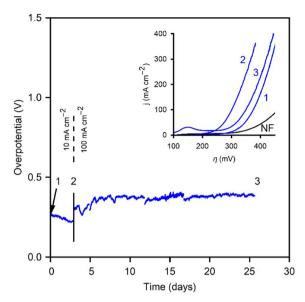
Fig. 9 CP curves of a CoNF electrode for 10 mA cm $^{-2}$  (up to the black line) and 100 mA cm $^{-2}$ . Numbered points where the LSVs are taken are noted. Inset: polarization curves for the bare ANF and the three CoANF points noted in the CP curves.
