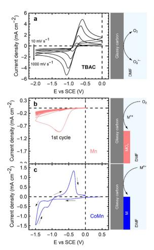
Fig. 1 Current density vs. potential cycles of a GCE in DMF with: (a)  $0.1 \, \text{M}$  TBAC, saturated with oxygen, at scan rates of 10 mV s<sup>-1</sup>, 100 mV  $s^{-1}$ , 500 mV  $s^{-1}$ , 1000 mV  $s^{-1}$ . (b) 0.1 M MnCl<sub>2</sub> saturated with oxygen, at 50 mV s<sup>-1</sup>. (c) 0.05 M CoCl<sub>2</sub>, 0.05 M MnCl<sub>2</sub>, de-oxygenated, at 50 mV s<sup>-1</sup>. Sketches of the respective processes accompany the curves.
