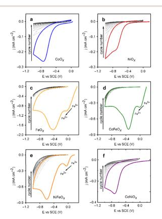
Fig. 3 Cyclic voltammograms at 20 mV s<sup>-1</sup> of the deposition of the single (Ni, Co, Fe) and mixed (CoFe, NiFe, CoNi) metal oxides over 20 cycles. Potential regions for the electrochemical reactions discussed are noted. The cycle number increases from each initial cycle highlighted, to the subsequent cycles trending towards 0 current. (a) Co. (b) Ni. (c) Fe. (d) CoFe. (e) NiFe. (f) CoNi.
