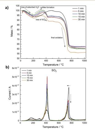
Fig. 4 Relative mass loss during TG-MS measurements in air for Ni<sub>2</sub>FeS<sub>4</sub> obtained after different synthesis durations (a) and SO<sub>2</sub> evolution detected by MS depending on the temperature (b).
