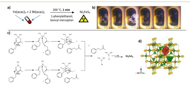
Fig. 1 General reaction equation for the formation of  $Ni_2FeS_4$  (a), photographs of observed light flashes and nanosheet formation (b), reaction sequence based on a nucleophilic attack of benzyl mercaptan similar to what was reported for alcohols (c) and crystal structure (d).
