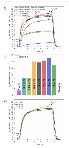
Fig. 6 H<sub>2</sub> evolution over P25 loaded with different amounts of Ni<sub>2</sub>FeS<sub>4</sub> under 1 sun simulated sunlight (a and b). Additionally, the H<sub>2</sub> evolution for 5 wt% Ni<sub>2</sub>FeS<sub>4</sub>@P25, with Ni<sub>2</sub>FeS<sub>4</sub> obtained after different synthesis durations in the microwave is shown (c). The lamp was switched on after 30 min and turned off after 5 h of irradiation
