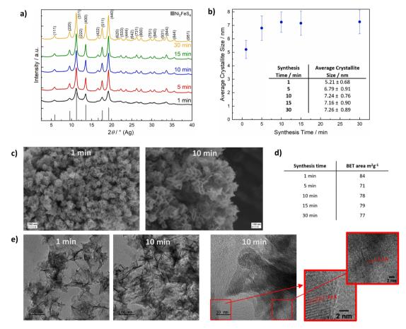
Fig. 2 XRD patterns for Ni<sub>2</sub>FeS<sub>4</sub> obtained after different synthesis times (a), corresponding crystallite sizes as determined by the integral breadth method (b), SEM images of Ni<sub>2</sub>FeS<sub>4</sub> nanosheets obtained after 1 and 10 min (c) and BET surface areas (d). For the identification of reflections, the ICDD reference card 00-047-1740. Additionally, TEM images of Ni₂FeS₄ nanosheets obtained after 1 and 10 min are shown in (e).
