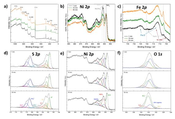
Fig. 3 XP spectra for Ni<sub>2</sub>FeS<sub>4</sub> obtained after different synthesis durations. Survey scan (a), Ni 2p spectra normalised to the Ni-S peak for qualitative comparison (b), normalised Fe 2p spectra (c), as well as fitted S 2p (d), Ni 2p (e) and O 1s spectra (f).
