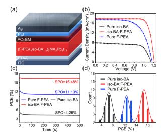
Fig. 4 (a) Device architecture of our Q-2D PSCs. (b) J-V curves, (c) steady-state PCEs at the maximum power point, (d) PCE histograms for 20 devices of pure iso-BA, iso-BA;F-PEA and pure F-PEA based PSCs.
