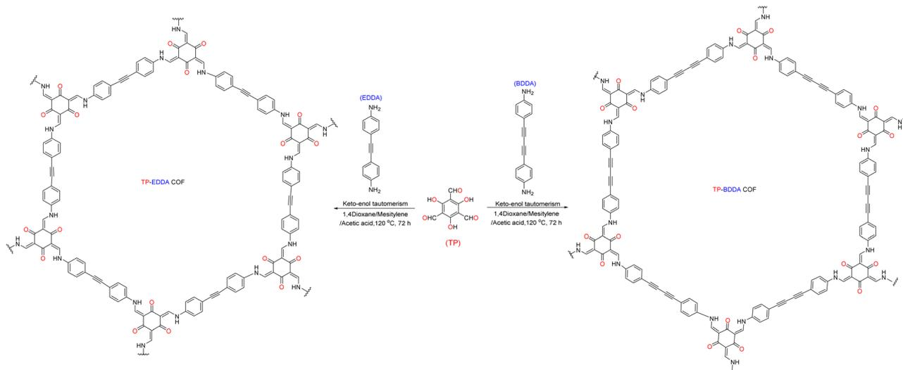
Fig. 5 Synthesis of TP-EDDA and TP-BDDA COFs.
