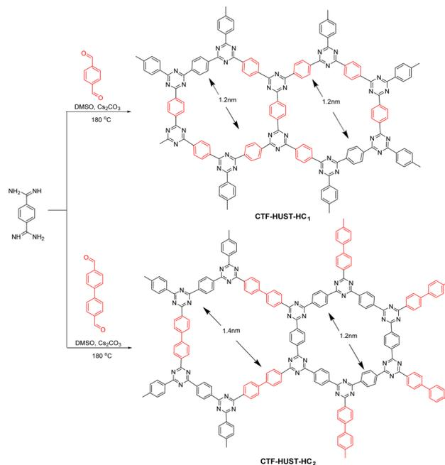
Fig. 15 Synthesis of CTF-HUST-HC<sub>1</sub> and CTF-HUST-HC<sub>2</sub>.
