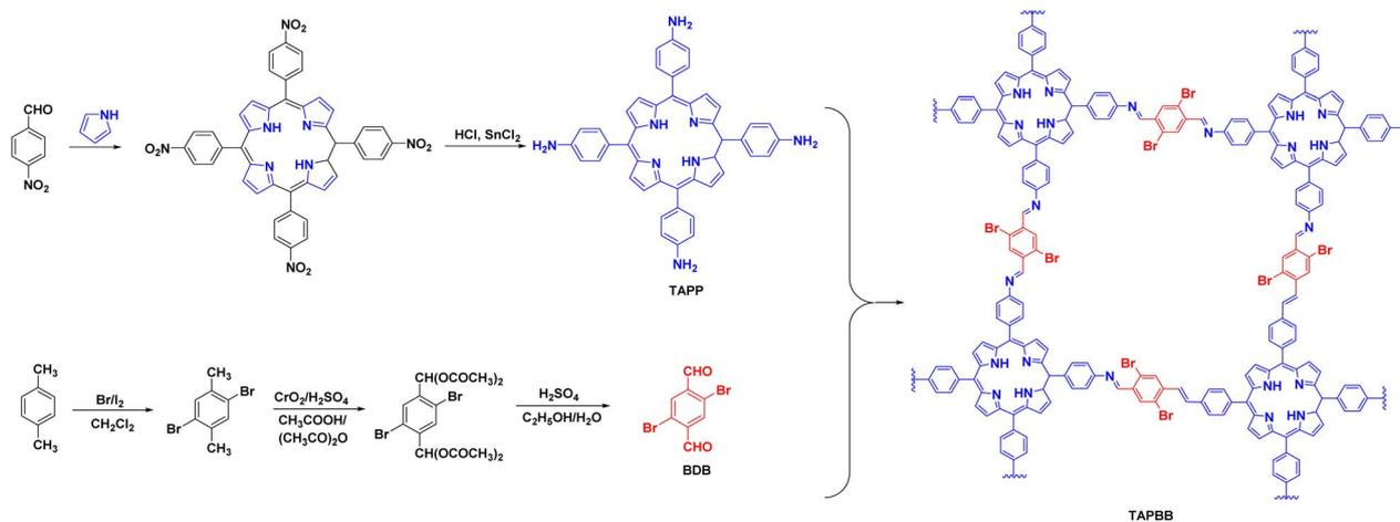
Fig. 9 Synthesis route of TAPBB-COF.
