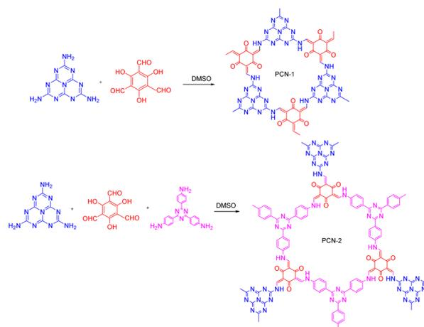
Fig. 13 Synthesis route of PCN-1 and PCN-2.
