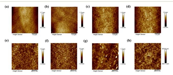
Fig. 5 Atomic force microscopy (AFM) images of (a and e) the recycled Pd electrode surface; (b and f) commercial Pd electrode surface; PCBM thin films on Pd e-beam evaporated electrodes from (c and g) recycled Pd, (d and h) commercial Pd. 5  $\mu$ m  $\times$  5  $\mu$ m  $\times$  5  $\mu$ m sized images (a–d), and 2  $\mu$ m  $\times$  2  $\mu$ m-sized images (e-h).
