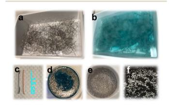
Fig. 1 Pd peeling from waste wires. (a) Pd plated waste wire in the open reaction vessel. (b) Reaction environment after 30 m at room temperature. (c) Pristine and peeled wires after a 6 h-long process. (d) Gooch vacuum filtration. (e) Dried and recovered Pd. (f) Pd peeled flakes
