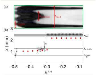
Fig. 4 (a) Hierarchical wrinkling within the smallest repeating unit of the "alternating folds" pattern, identified by the green box in Fig. 3, aligned with (b) the corresponding axial wavelength  $\lambda$ , plotted as a function of the cross-channel coordinate y; data in (b) is obtained from experiments (stars) and the FvK model (diamonds)
