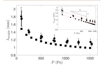
Fig. 6 The initial wrinkling wavelength,  $\lambda_{\text{wrinkle}}$ , as a function of the pressure P in experiments (circle) and numerical simulations (square). The inset shows the same data on a log-log scale with lines corresponding
