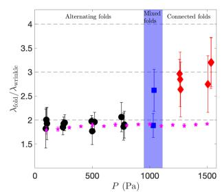
Fig. 9 The wavelength ratio  $\lambda_{\rm fold}/\lambda_{\rm wrinkle}$  as a function of the pressure P for different types of coarsened patterns obtained experimentally, and the alternating folds obtained numerically (stars).
