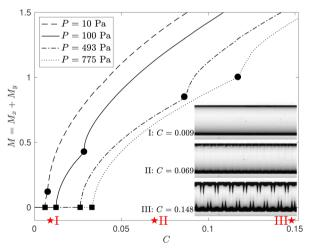
Fig. 7 The combined norm,  $M = M_x + M_y$ , where  $M_x$  and  $M_y$  are defined in eqn (11) and (12), respectively, as a function of the level of swelling, C, for four different pressures, P. The onset of wrinkling and the secondary symmetry-breaking instability are identified by square and circular markers, respectively. The insets show experimental images at P = 775 Pa for three values of C, as marked with stars on the C-axis.
