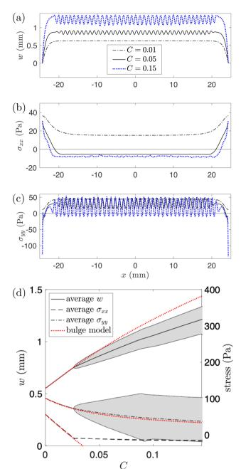
Fig. 5 (a) The deflection,  $w_r$  (b) the axial stress,  $\sigma_{xx_r}$  and (c) the crosschannel stress,  $\sigma_{vv}$  along the channel centreline (y = 0) for P = 493 Pa and varying C. (d) The average (computed over the central part of the channel,  $|x| < L/2 - \delta$ ) of the same three quantities, with lighter lines indicating the minimum/maximum of the relevant quantity with the range shaded. Corresponding predictions from the bulge model are shown with red dotted lines.
