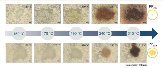
Fig. 6 In situ optical microscopy of polypropylene (PP) cracking using FCC catalyst. Individual polymer grains were placed on a bed of FCC catalyst and heated at 10 °C min<sup>-1</sup> under  $N_2$  flow in a Linkam stage. Images were acquired every minute. See ESI† for videos of the full reaction. Top:  $PP_{23k}$ . Bottom:  $PP_{307k}$ .
