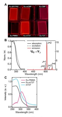
Fig. 3 Optical properties of  $Eu(hfa)_3(TPPO)_2$ -doped films. (A) Photos of emission from the fabricated films upon photoexcitation with 254 nm. (B) Absorption (solid line), excitation probed at 615 nm (broken line), and emission (red line) spectra of the Eu-mT2T film. (C) Absorption spectra of the Eu-PMMA film (pink line), Eu-mT2T film (black line), and mT2T neat film (sky blue line).
