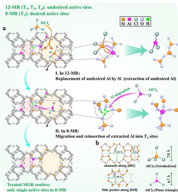
Fig. 10 (a) Schematic of a typical treatment process, showing the directional migration of framework Al into T<sub>3</sub> sites of the MOR zeolite via LPST. (b) Topology of MOR and steric configuration of SiCl<sub>4</sub> and AlCl<sub>3</sub> molecules with a kinetic diameter of 7.0 and 6.7 Å, respectively. Reproduced from ref. 203 with permission from Wiley, Copyright 2022.
