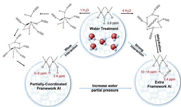
Fig. 4 Proposed mechanism of the dealumination process induced by hydrothermal-treatment of SSZ-13 zeolite. Reproduced from ref. 137 with permission from the Royal Society of Chemistry, Copyright 2022.
