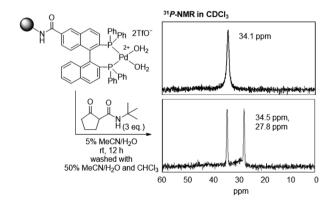
Fig. 3 <sup>31</sup>P-NMR analysis of TentaGel-supported Pd agua complexes before and after mixing with β-ketoamide.
