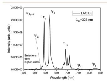
Fig. 5 Emission spectrum of LAO:Eu phosphor when excited at  $325 \ \text{nm}$ .
