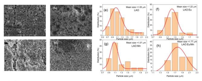
Fig. 3 (a-d) Morphological SEM images of the prepared (a) LAO, (b) LAO:Eu, (c) LAO:Mn and (d) LAO:Eu/Mn and (e-h) particle size distribution based on the SEM images, respectively.
