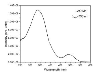
Fig. 6 Excitation spectrum of LAO:Mn phosphor monitoring emission at 736 nm radiation
