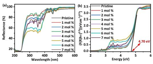
Fig. 2 (a) Diffusive reflectance spectra for  $Ba(La_{2-x}Dy_x)ZnO_5$  (x = 0-7 mol%) phosphor (b) Tauc's plot for estimating the indirect bandgap of synthesized phosphor materials.
