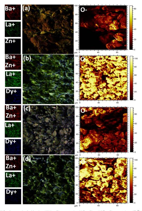
Fig. 5 TOF-SIMS surface mapping for (a) undoped (b) 1 mol%, concentrations (c) 5 mol%, and (d) 7 mol% concentations of Dy $^{3+}$  in Ba(La $_{2-x}$ Dy $_x$ ) ZnO $_5$  phosphor.
