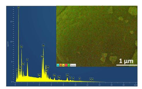
Fig. 4 EDS spectrum for 5 mol% doped BaLa<sub>2</sub>ZnO<sub>5</sub> coated with Iridium
