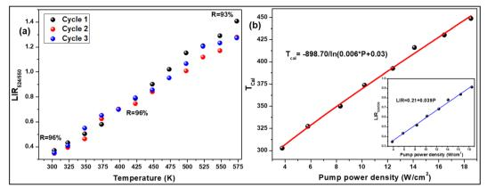
Fig. 5 (a) Repeatability of LIR from 300 K to 573 K for 3 cycles, (b) a plot of calculated temperatures vs. pump power densities (inset: LIR vs. pump power densities) for 7 mol%  $Er^{3+}$ -10 mol%  $Yb^{3+}$ : Na $Zr_2(PO_4)_3$  phosphors.
