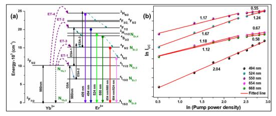
Fig. 3 (a) Energy level diagram of Er<sup>3+</sup>-Yb<sup>3+</sup> codoped system, (b) In-In plot of UC emission intensity and laser pump power density.
