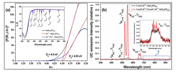
Fig. 2 (a) Tauc plot of  $Er^{3+}/Er^{3+}-Yb^{3+}:NaZr_2(PO_4)_3$  phosphors, (inset: diffuse reflectance spectra of 7 mol%  $Er^{3+}$  and 7 mol%  $Er^{3+}-10$  mol%  $Yb^{3+}:NaZr_2(PO_4)_3$  phosphors. (b) UC emission spectra of 7 mol%  $Er^{3+}-10$  mol%  $Yb^{3+}:NaZr_2(PO_4)_3$  phosphors and the inset shows the enlarged spectra of (804, 824) nm peak.
