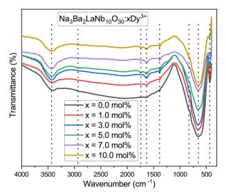
Fig. 8 Fourier transformed infrared (FT-IR) spectrum of Na<sub>3</sub>Ba<sub>2</sub>- $LaNb_{10}O_{30}:xDy^{3+}$  (x = 0, 1, 3, 5, 7 and 10 mol%) phosphor at room temperature.
