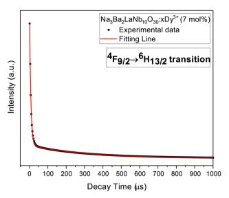
Fig. 18 Decay curve  $4F_{9/2} \rightarrow 6H_{13/2}$  transition in  $Na_3Ba_2LaNb_{10}O_{30}$ :- $xDy^{3+}$  (x=7 mol%) phosphor.
