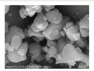
Fig. 4 FE-SEM micrograph of Na $_3$ Ba $_2$ LaNb $_{10}$ O $_{30}$ :xDy $^{3+}$  (x = 7 mol%) phosphor sintered at 1300 °C.
