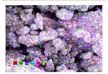
Fig. 6 Elemental mapping of  $Na_3Ba_2LaNb_{10}O_{30}$ : $xDy^{3+}$  (x=7 mol%) phosphor.
