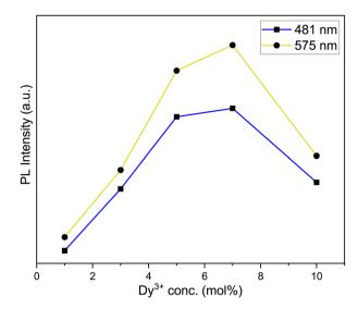
Fig. 13 Variation of emission intensity of the emission peaks to various  ${\rm Dy}^{3+}$  ions concentration.
