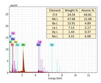
Fig. 5 EDX spectrum of  $Na_3Ba_2LaNb_{10}O_{30}:xDy^{3+}$  (x=7 mol%) phosphor.
