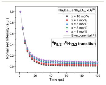
Fig. 19 Decay curves for  $4F_{9/2} \rightarrow 6H_{13/2}$  transition in Na<sub>3</sub>Ba<sub>2</sub>LaNb<sub>10</sub>-O<sub>30</sub>:xDy<sup>3+</sup> ( $x=1,\,3,\,5,\,7$  and 10 mol%) phosphors.
