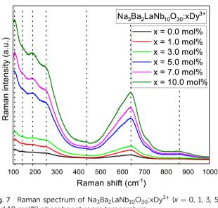
Fig. 7 Raman spectrum of  $Na_3Ba_2LaNb_{10}O_{30}:xDy^{3+}$  (x = 0, 1, 3, 5, 7and 10 mol%) phosphor at room temperature.
