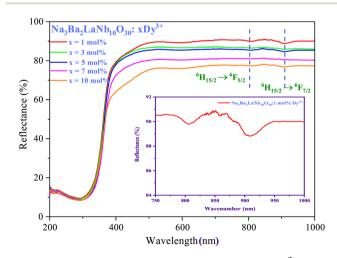
Fig. 9 Diffuse reflectance spectra of Na<sub>3</sub>Ba<sub>2</sub>LaNb<sub>10</sub>O<sub>30</sub>:xDy<sup>3+</sup> (x = 1, 3,5, 7 and 10 mol%) phosphor.
