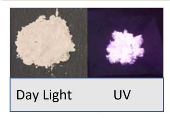
Fig. 1 Image of Na<sub>3</sub>Ba<sub>2</sub>LaNb<sub>10</sub>O $_{30}$ :xDy<sup>3+</sup> (x=7 mol%) phosphor sample under daylight and 365 nm UV light.
