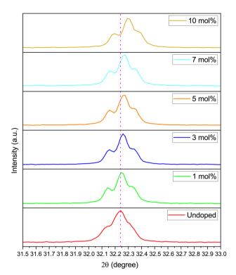
Fig. 3 XRD peak corresponding to 311 plane of  $Na_3Ba_2LaNb_{10}O_{30}$ :- $xDy^{3+}$  (x=0,1,3,5,7 and 10 mol%) phosphors.
