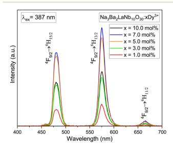
Fig. 12 PL emission spectra of  $Na_3Ba_2LaNb_{10}O_{30}$ :xDy $^{3+}$  (x=1, 3, 5, 7 and 10 mol%) phosphors under the excitation wavelength of 387 nm.
