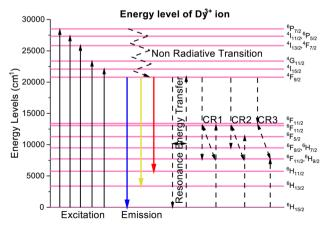
Fig. 15 Partial energy level diagram of  $\mathrm{Dy}^{3+}$  in  $\mathrm{Na_3Ba_2LaNb_{10}O_{30}}$  phosphor.
