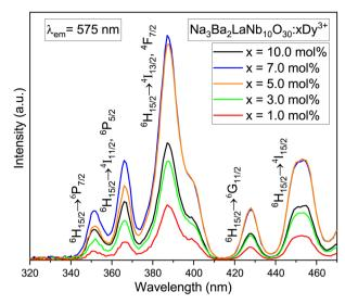
Fig. 11 PLE spectra of  $Na_3Ba_2LaNb_{10}O_{30}:xDy^{3+}$  (x=1, 3, 5, 7 and 10 mol%) phosphors by fixing emission at 575 nm.
