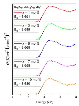
Fig. 10 Tau plot of un-doped and  $Na_3Ba_2LaNb_{10}O_{30}$ :xDy<sup>3+</sup> (x = 1, 3, 5, 7 and 10 mol%) phosphors for the determination of optical bandgap  $E_g$  (assuming indirect transitions).
