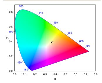
Fig. 16 CIE 1931 chromaticity diagram showing the color coordinates of  $Na_3Ba_2LaNb_{10}O_{30}$ :xDy<sup>3+</sup> (x=1, 3, 5, 7 and 10 mol%) phosphors.
