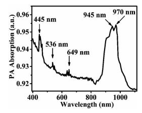
Fig. 8 The PA absorption spectrum in 400–1200 nm range for sample annealed at 1000 °C.
