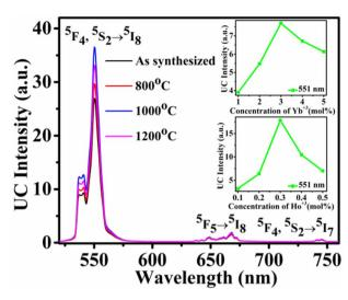
Fig. 4 Upconversion emission spectra for as-synthesized  $\vartheta$  annealed samples in 520–760 nm range. The inset (up) shows the intensity variation for different Yb<sup>3+</sup> ion concentrations and inset (down) shows intensity variation for different Ho<sup>3+</sup> ion concentrations.
