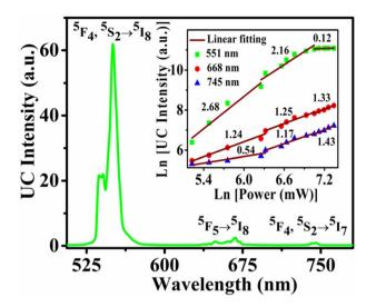
Fig. 5 (a) The UC spectrum of the optimized sample at the excitation power of 1150 mW. Inset plot shows the ln(P) vs.  $ln(I_{UC})$  plots for different emission bands.
