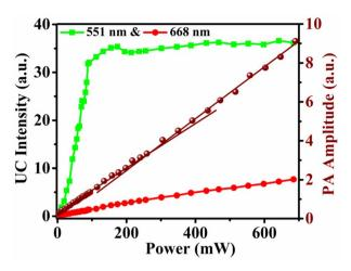
Fig. 6 Variation of UC emission intensity of 551 nm, & 668 nm bands and PA signal amplitude with excitation pump powers for the sample annealed at 1000 °C for 2 h. PA signal is on right Y-axis.
