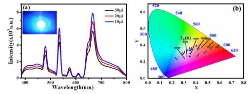
Fig. 7 (a) EL spectrum of the WLEDs with distinct thickness of the CQDs +  $Tb^{3+}$  (25%). Inset: WLEDs demonstration. (b) CIE chromaticity plot for the WLEDs at various molar concentration of Tb<sup>3+</sup> ions (0%, 5%, 15%, and 25%)
