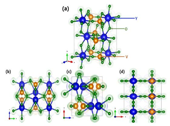
Fig. 2 Crystal structure of YVO<sub>4</sub> (a) standard orientation and (b-d) three different orientations 100, 010, and 001.
