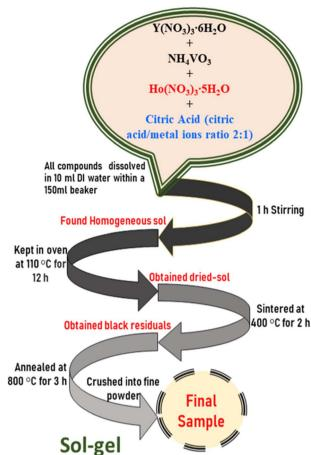
Fig. 1 Flow chart of synthesis method of  $Y_{1-x}VO_4:xHo^{3+}$  phosphors.
