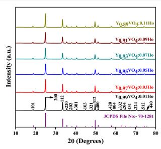
Fig. 3 Powder XRD patterns of  $Y_{1-x}VO_4:xHo^{3+}$  phosphors.
