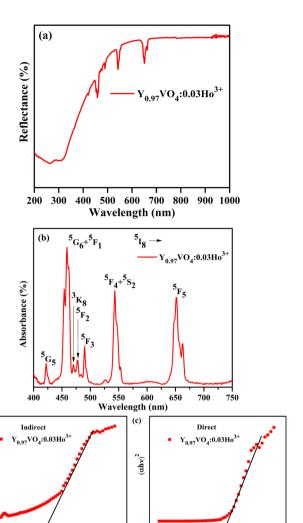
Fig. 6 (a) Diffuse reflection spectrum, (b) absorption spectrum and (c) plots of indirect and direct bandgaps of  $Y_{0.97}VO_4$ : 0.03Ho<sup>3+</sup> phosphor.
