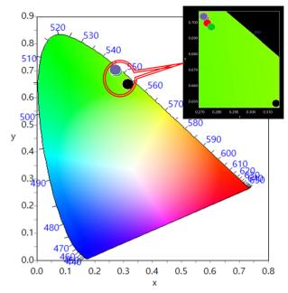
Fig. 10 CIE diagram for  $Y_{1-x}VO_4:xHo^{3+}$  phosphors.
