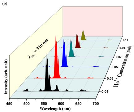
Fig. 7 Photoluminescence spectra of  $Y_{1-x}VO_4$ : $xHo^{3+}$  phosphors: (a) excitation spectra ( $\lambda_{emi} = 541$  nm) and (b) emission spectra ( $\lambda_{exc} = 310$  nm).
