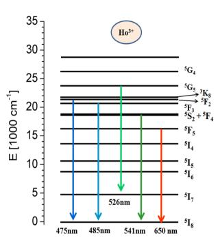
Fig. 8 Schematic energy level diagram of Ho<sup>3+</sup> ion.
