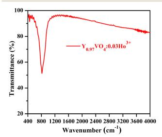
Fig. 5 FT-IR spectrum of Y<sub>0.97</sub>VO<sub>4</sub>:0.03Ho<sup>3+</sup> phosphor.
