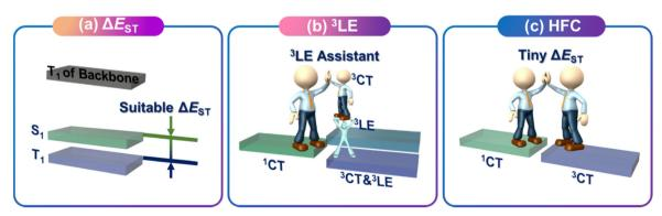
Fig. 1 The rules governing the excited state properties of conjugated polymer TADF. (a) Maintaining suitable  $\Delta E_{ST}$ ; (b) localized triplet excited state assisted reverse intersystem crossing; (c) hyperfine coupling facilitates reverse intersystem crossing.
