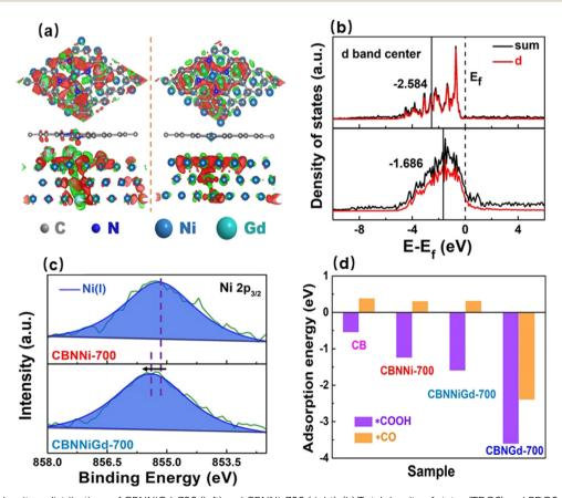
Fig. 5 (a) Charge-density redistributions of CBNNiGd-700 (left) and CBNNi-700 (right). (b) Total density of states (TDOS) and PDOS of Ni 3d and (c) XPS high-resolution Ni 2p3/2 spectra of CBNNi-700 (upper) and CBNNiGd-700 (lower). (d) Adsorption energies of \*CO and \*COOH for various electrocatalysts.<sup>116</sup> Reproduced with permission from Wiley-VCH Verlag GmbH & Co. KGaA, copyright 2022.
