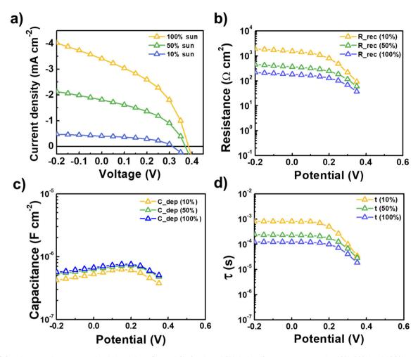
Fig. 5 (a) Steady-state photocurrent densities of the w/o-seed Sb<sub>2</sub>Se<sub>3</sub>-based PV during IS measurement under 10%, 50%, and 100% sun illumination. (b) Resistances, (c) capacitance, and (d) time constants for the charge transfer of w/o-seed Sb<sub>2</sub>Se<sub>3</sub> PV from the IS fitting procedure.
