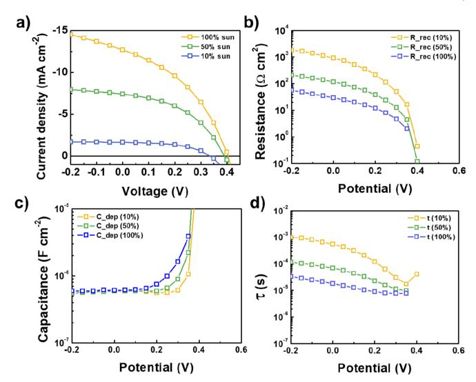
Fig. 3 (a) Steady-state photocurrent densities obtained by the w-seed Sb<sub>2</sub>Se<sub>3</sub> PV during IS measurement under 10%, 50%, and 100% sun illumination. (b) Resistances (c) capacitance, and (d) time constants for charge transfer of the w-seed Sb<sub>2</sub>Se<sub>3</sub> PV from the IS fitting procedure.
