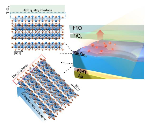
Fig. 6 Schematic illustration of the proposed novel bilayer  $Sb_2Se_3$  configuration that can effectively transport the charge carriers without recombination and also form a high quality interface with the  $TiO_2$  layer.
