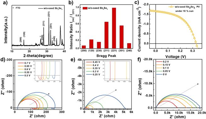
Fig. 4 (a) Diffraction patterns and (b) peak intensities ratio  $(I_{(lnk)}/I_{(221)})$  of the obtained w/o-seed Sb<sub>2</sub>Se<sub>3</sub> films (c) J-V behavior exhibited by the w/o-seed Sb<sub>2</sub>Se<sub>3</sub> PV under 10% sun illumination. (d-f) Nyquist plots of the w/o-seed Sb<sub>2</sub>Se<sub>3</sub> PV at the designated applied potential.
