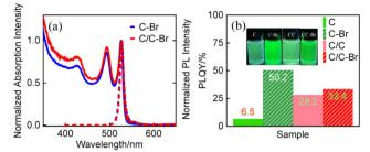
Fig. 5 (a) Normalized absorption and PL spectra of C and C/C NPLs after 5 h of ligand exchange. (b) PLQYs before and after ligand exchange for C and C/C NPLs. Insets: images of the samples before and after ligand exchange under UV light illumination.
