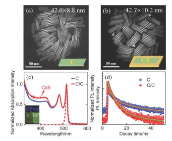
Fig. 1 STEM image of (a) C, (b) C/C NPLs. Insets are the schematic diagrams of their corresponding structures. (c) Normalized UV-visible absorption and PL spectra of C and C/C NPLs. Inset is the image of samples under UV light illumination. (d) Room temperature TRPL of C and C/C NPLs.
