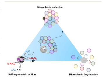
Fig. 1 Schematic illustration of our current photocatalytic micromotorbased system (at center) combining the principles of inherently selfasymmetric motion (bottom left), micromotor-based collection of microplastic (top), and photocatalytic degradation of microplastics (bottom right). The colorful translucent spheres represent polystyrene microparticles, and the transparent ones close to the photocatalyst (right and center) are degraded due to the photocatalytic action.
