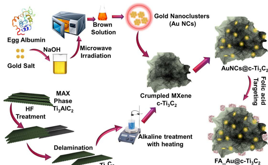
Scheme 1 Synthesis procedure of the folic acid conjugated MXene gold composite (FA_Au@c-Ti 3 C 2 ).
