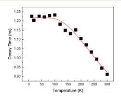
Fig. 3 Temperature dependence of the ZPL time constant  $\tau$  at  $\approx$ 740 nm. The solid red line is the fit – see text.
