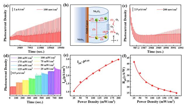
Fig. 7 (a) Long cycling stability measurement in a low oxygen environment, (b) OSPC mechanism, (c) long cycling stability measurement in enough oxygen environment, (d) light intensity-dependent photocurrent density, and (e)  $I_{\rm ph}$  and (f)  $R_{\rm ph}$  values extracted from (d).
