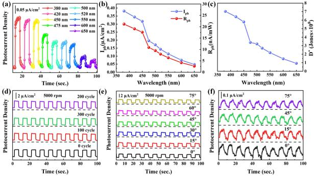
Fig. 8 (a) Photocurrent density, (b) the calculated Iph and Rph, and (c) specific detectivity (D\*) values under different wavelengths; flexibility measurement with (d) different bending cycles and (e) bending angles in the PEC-type photodetector; (f) flexibility measurement in various bending angles in a solid photodetector
