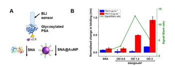
Fig. 4 (A) Schematic comparison of lectin vs. lectin@AuNP conjugates BLI response in the (B) presence of PSA (0.4  $\mu g$  mL<sup>-1</sup>) and absence of PSA (negative control). Other experimental conditions: SNA 50  $\mu$ g mL<sup>-1</sup>; SNA@AuNP (coated with SNA 50  $\mu$ g mL<sup>-1</sup>). Error =  $\pm$  S.D.
