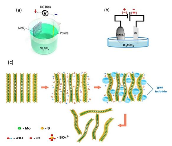
Fig. 7 (a) Schematic illustration of the experimental setup for the anodic electrochemical exfoliation of bulk  $MoS_2$  crystal. (b) Schematic diagram of the electrochemical setup for exfoliation of natural  $MoS_2$  crystals. (c) Schematic illustration of the electrochemical exfoliation mechanism. Adapted with permission from ref. 65 (ACS Nano, 2014, 8(7), 6902–6910) Copyright (2014) American Chemical Society.
