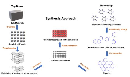
Fig. 1 Schematic representation of the synthesis approach.
