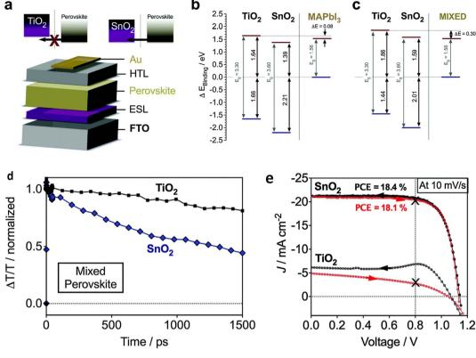
Fig. 21 (a-c). Diagram of energy level plans and electron inoculation properties of SnO<sub>2</sub>- and TiO<sub>2</sub>-based planar PSCs, (d) transient absorption findings, (e) current-voltage (J-V) curves of  $TiO_2$ - and  $SnO_2$ -based planar mixed halide-mixed cation PSCs (reproduced with permission from ref. 184. Copyright 2015 RSC)
