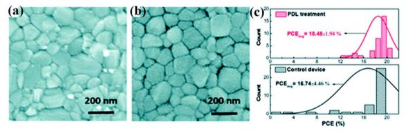
Fig. 31 SEM top view pictures of perovskite thin layers (a) without any treatment and (b) with post-device ligand treatment. (c) Histograms of the device efficiencies with PDL treatment and without any treatment (37 cells were made-up and verified, reproduced with permission from ref. 225. Copyright 2018 Elsevier).
