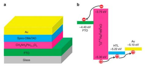
Fig. 5 (a) Symbolic representation of the ETL-free planar PSC arrangement and (b) energy level illustration of the planar PSC presenting gathering and parting of photo-generated electrons and holes in the absence of ETL (reproduced with permission from ref. 48, copyright 2015 NPG).
