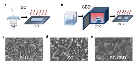
Fig. 22 Symbolic diagram showing the preparation of SnO<sub>2</sub> thin layers using (a) spin coating (SC) and (b) chemical bath deposition (CBD). (c) Top-view SEM pictures of SnO<sub>2</sub> films prepared by atomic layer deposition (ALD), (d) spin coating (SC), and (e) spin coating and chemical bath deposition (SC-CBD). All scale bars are 200 nm (reproduced with permission from ref. 74. Copyright 2016 RSC).
