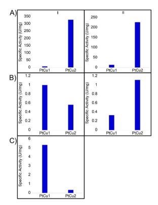
Fig. 6 Catechol oxidase-like activity of different Pt catalysts by oxidation of L-DOPA under different conditions at room temperature expressed in values of specific activity (U per mg Pt). (I) room temperature, (II) 50 °C. (A) Buffer sodium phosphate pH 7; (B) 40:60 ACN: H<sub>2</sub>O; (C) 30: 70 dioxane: H<sub>2</sub>O.
