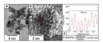
Fig. 5 (a) HRTEM image of PtCu2, (b) representative lattice fringe under higher magnification and (c) determination of the inter-planar distance using a plot profile.
