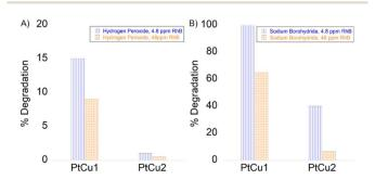
Fig. 9 Degradation of rhodamine B (A) in the presence of  $H_2O_2$  and (B) in the presence of NaBH<sub>4</sub>. 4.8 ppm of RhB (blue column), 48 ppm of RhB (orange column).
