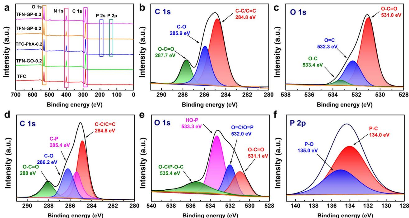
Fig. 3 (a) XPS survey spectra of TFC and TFN composite membranes; (b) C 1s and (c) O 1s XPS spectra of the TFN-GO-0.2 membrane; (d) C 1s, (e) O 1s, and (f) P 2p XPS spectra of the TFN-GP-0.2 membrane.
