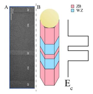
Fig. 4 (A) High-resolution transmission electron micrograph of an InAs NW with a ZB QD sandwiched between WZ barriers. (B) Schematic representation of the crystal structure stacking sequence and the resulting type-II band alignment. Adapted from Fig. 1 by Potts, H., Chen, I., Tsintzis, A. et al., Electrical control of spins and giant g-factors in ring-like coupled quantum dots, Nat. Commun., 10, 5740, (2019), https://doi.org/10.1038/s41467-019-13583-7 Is licensed under CC BY 4.0.
