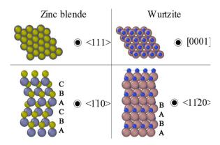
Fig. 2 The atomic arrangement for the ZB and WZ structures.
