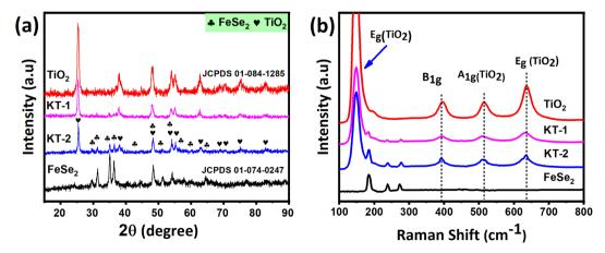
Fig. 1 (a) Crystal structure and (b) vibrational modes of the  $FeSe_2$ ,  $TiO_2$ , KT-1, and KT-2 composite.
