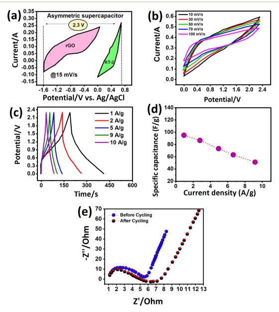
Fig. 8 Energy storage characteristics of KT-2//AC asymmetric faradaic SC, (a) CV curves at different potential frames, (b) CV curves at 2.3 V, (c) charge profiles at different rates, (d) decay in capacitance w.r.t current, (e) impedance plots.
