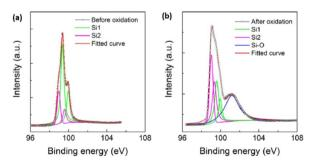
Fig. 10 Si 2p core level XPS spectra of epitaxial silicene on Ag(111) before (a) and after (b) exposure to 600 L of oxygen. Si1 and Si2 represent Si-Ag and Si-Si, respectively. The silicence layer is oxidized It can be noted that the intensity of the peaks related to Si-Ag bonds has significantly decreased after oxygen exposure. Adapted with permission from ref. 182, Springer Nature.
