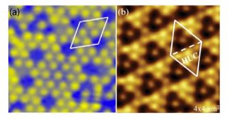
Fig. 12 STM images of the  $2(\sqrt{3}\times2\sqrt{3})R30^\circ$  (a) and  $(4\times4)$  Si/Ag(111) reconstruction (b) after hydrogen exposure. In (a) the rhombus corresponds to the pristine  $2(\sqrt{3}\times2\sqrt{3})R30^\circ$  unit cell, while in (b) it corresponds to a shift of the pristine  $(4\times4)$  unit cell. Adapted with permission from ref. 66, Copyright 2015 by the American Physical Society and with permission from ref. 81, Copyright 2015 American Chemical Society.
