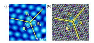
Fig. 13 (a) STM image of K atoms adsorbed on silicene/Ag(111) at 200 K. The image shows a boundary between three equivalent domains rotated by  $\pm 120^\circ$ . (b) Structural atomic model proposed. Adapted with permission from ref. 197, Copyright 2022 by the American Physical Society.
