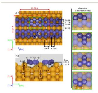
Fig. 6 Structural model for the silicon NRs on Au(110) proposed from the fit of XPD data in top view (a) and side view (b). Reprinted from ref. 132, Copyright 2019, with permission from Elsevier.
