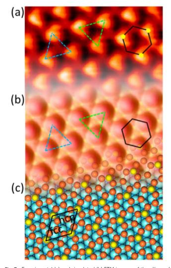
Fig. 7 Experimental (a) and simulated (b) STM images of the silicene/ Ir(111) system. (c) Top view of the relaxed atomic model of the  $(\sqrt{3} \times \sqrt{3}\,)$  silicene/ $(\sqrt{7} \times \sqrt{7}\,)$  Ir(111) configuration. Adapted with permission from ref. 16, Copyright 2013 American Chemical Society.
