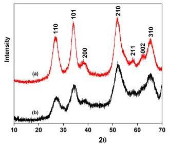
Fig. 1 XRD spectra of (a) SnO<sub>2</sub> NPs in a powder form and (b) SnO<sub>2</sub> NPs encapsulated within SA beads.
