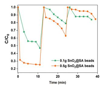
Fig. 12 Regenerative studies of 0.5 g and 0.1 g SnO $_2$ @SA beads for 5  $\mu$ M CR aqueous solution.
