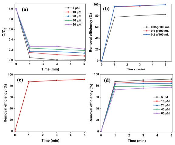
Fig. 6 (a) Adsorption efficiencies of spherical SnO<sub>2</sub> NPs as observed for various dye concentrations; (b) effect of adsorbent dosage on the removal efficiency for 5  $\mu$ M CR at pH = 5; (c) effect of contact time upon the removal efficiency for 5  $\mu$ M CR dye; and (d) effect of dye concentration on the removal efficiency for CR by 0.1 g/100 mL of SnO<sub>2</sub> NPs.
