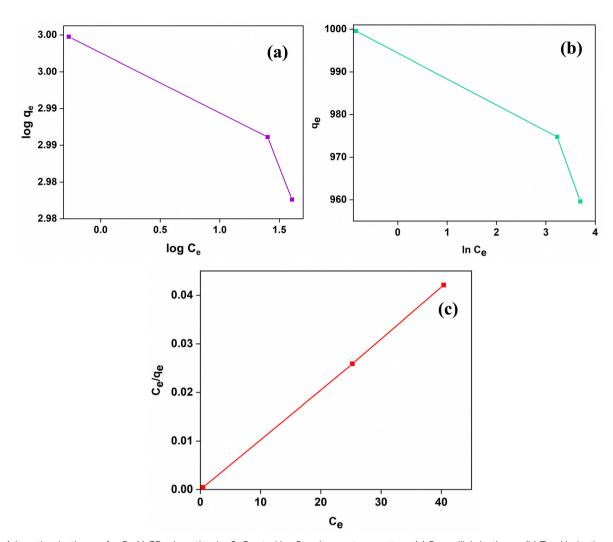
Fig. 9 Adsorption isotherms for 5  $\mu$ M CR adsorption by SnO<sub>2</sub> at pH = 5 and room temperature. (a) Freundlich isotherm, (b) Temkin isotherm and (c) Langmuir isotherm.
