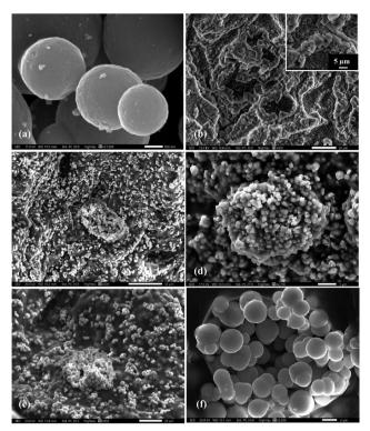
Fig. 3 SEM images of (a) SnO<sub>2</sub> NPs and (b) SA beads crosslinked by CaCl<sub>2</sub> at 20  $\mu$ m, with the inset representing the image taken at 5  $\mu$ m; panels (c), (d), (e) and (f) show 0.5 g SnO<sub>2</sub> encapsulated within SA beads at different magnification.
