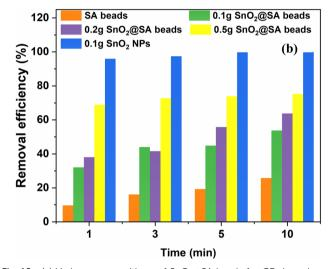
Fig. 10 (a) Various compositions of SnO<sub>2</sub>@SA beads for CR dye adsorption, and (b) their comparative analysis through a bar diagram.
