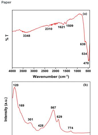
Fig. 2 (a) FTIR spectra and (b) Raman spectra of SnO<sub>2</sub> NPs.
