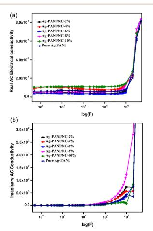
Fig. 4 (a) Real AC conductivity measurements with variation in applied frequency for NC doped Ag-PANI with 2, 4, 6, 8 and 10 wt%. (b) Imaginary AC conductivity measurements with variation in applied frequency for NC doped Ag-PANI with 2, 4, 6, 8 and 10 wt%
