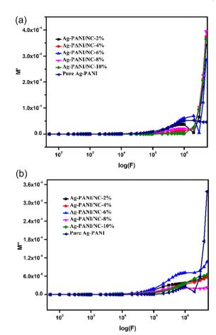
Fig. 6 (a) The real dielectric modulus M' of 2,4,6,8 and 10% Ag-PANI/NC composites as a function of applied frequency in the range of 50 Hz to 1 MHz. (b) The imaginary part of dielectric modulus M'' of 2,4,6,8 and 10% Ag-PANI/NC composites as a function of applied frequency in the range from 50 Hz to 1 MHz.
