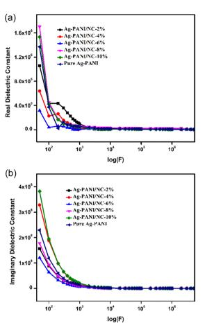
Fig. 5 (a) Variation in real dielectric constant *versus* function of applied frequency for 2, 4, 6, 8, and 10% Ag-PANI/NC composites. (b) Variation in imaginary dielectric constant *versus* function of applied frequency for 2, 4, 6, 8, and 10% Ag-PANI/NC composites.
