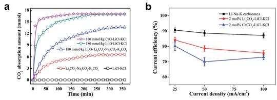
Fig. 6 (a) CO<sub>2</sub> absorption curves in different molten salts at 450 °C with the CO<sub>2</sub> partial pressure of 50 kPa; (b) current efficiency for galvanostatic electrolysis in different molten salts under CO<sub>2</sub> atmosphere at 450 °C.<sup>76</sup>
