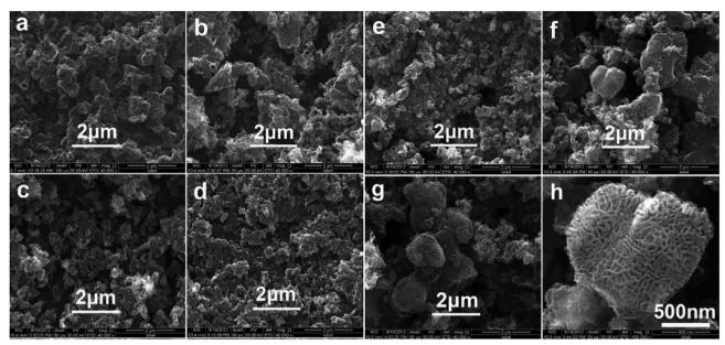
Fig. 14 SEM images of carbon powders obtained under cell voltages of 3.0 V (a), 3.5 V (b), 4.0 V (c), 4.5 V (d), 5.0 V (e), 5.5 V (f), (h) and 6.0 V (g) at  $450 \,^{\circ}$  C in  $\text{Li}_2\text{CO}_3$ -Na $_2\text{CO}_3$ -K2CO $_3$  mixture.
