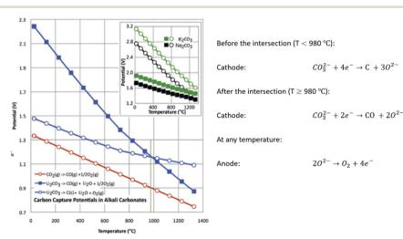
Fig. 5 Electrochemical conversion potential for carbon capture and conversion centra  $Li_2CO_3$  (main figure), or  $Na_2CO_3$  or  $K_2CO_3$  (figure inset); in the inset, squares refer to  $M_2CO_3 \rightarrow C + M_2O + O_2$  and circles to  $M_2CO_3 \rightarrow CO + M_2O + O_2$ . To the right of the brown vertical line, CO is preferred. And C is preferred to the left of the line.<sup>74</sup>
