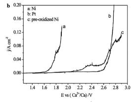
Fig. 11 (a) Polarization curves of metals in molten CaCl<sub>2</sub> - 2.5 mol% CaO at 850 °C (potential scan rate, 2 mV s<sup>-1</sup>); (b) polarization curves of Ni, Pt and pre-oxidized Ni in molten CaCl<sub>2</sub> at 850 °C (potential scan rate, 2 mV s<sup>-1</sup>). 103
