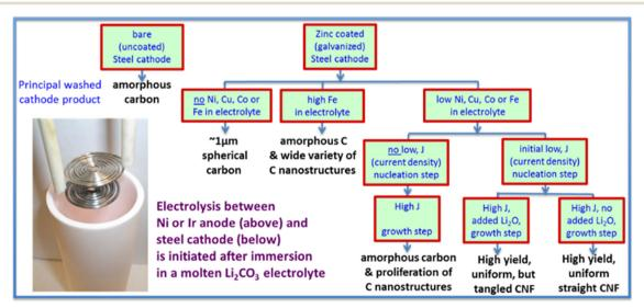
Fig. 8 Molten carbonate electrolysis pathways converting CO<sub>2</sub> leading to high yield, uniform CNF product.<sup>92</sup>
