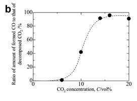
Fig. 16 (a) Amounts of decomposed CO2 gas and produced CO gas as a function of inlet gas flow rate; (b) ratio of the amount of formed CO gas to that of decomposed CO<sub>2</sub> gas as a function of the initial gas concentration of CO<sub>2</sub>. 42
