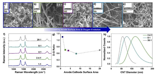
Fig. 12 Different anode to cathode surface area ratios (A:C) and the resulting carbon product using a Ni/Al<sub>2</sub>O<sub>3</sub> anode with 5 nm Fe on stainless steel cathode; a) 1:1, b) 2.4:1, c) 4:1, d) 8:1, e) 20:1 and f) Raman spectra, g) D:G ratio, and h) CNT diameter distribution at ratios of 2.4:1, 8:1, and 20:1.66
