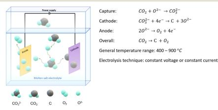
Fig. 4 A schematic of a molten salt electrochemical system towards carbon deposition.
