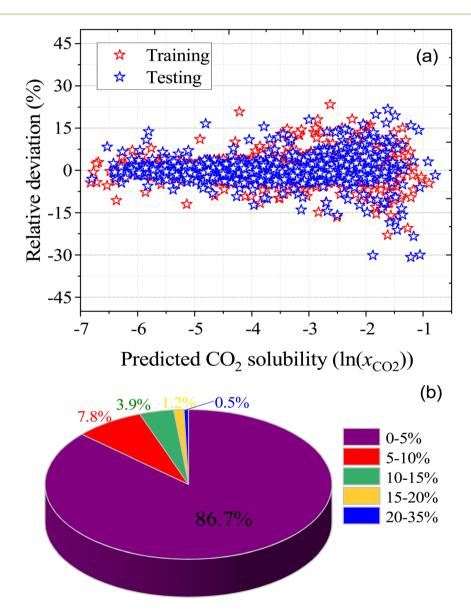
Fig. 7 (a) relative deviation between the experimental and predicted CO<sub>2</sub> solubilities in DES, and (b) the distribution of the absolute relative deviation in different deviation ranges.
