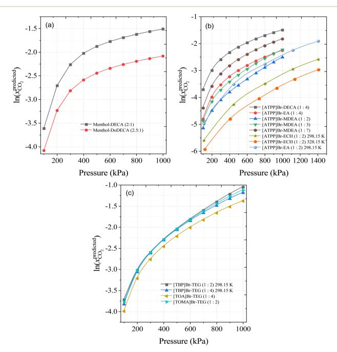
Fig. 12 Development of new DESs combination for improving CO<sub>2</sub> solubilities using the machine learning model, DES composed of (a) menthol as HBA and decanoic acid and dodecanoic acid as HBDs, (b) [ATTP]Br HBA and EA, DECA, MDEA, and ECH are HBDs, and (c) [TBP]Br, [TOA]Br, and [TOMA]Br are HBAs with TEG HBD.
