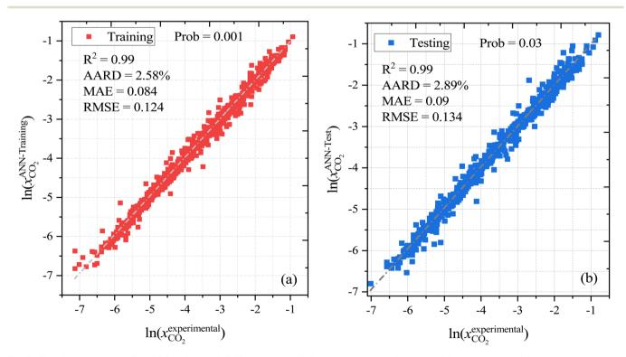
Fig. 6 Experimental and predicted CO<sub>2</sub> solubility in DESs using an ANN-based machine learning model (a) training set and (b) testing set.
