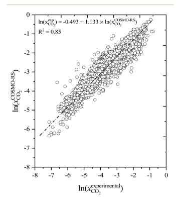
Fig. 4 Correlation between the COSMO-RS predicted and experimental CO<sub>2</sub> solubility in deep eutectic solvents.
